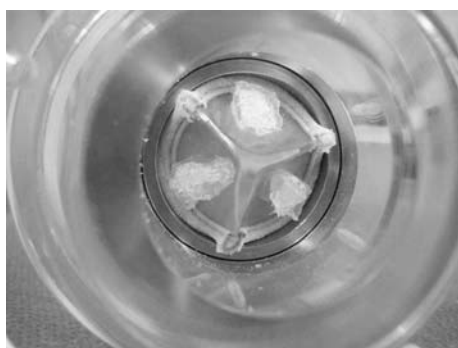
Fig. 6 Test specimen fixed in stainless steel tube
