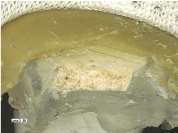
Fig. 8 Cutting result of moderately calcified bioprosthesis: Zoom (×20) on artificial calcification
